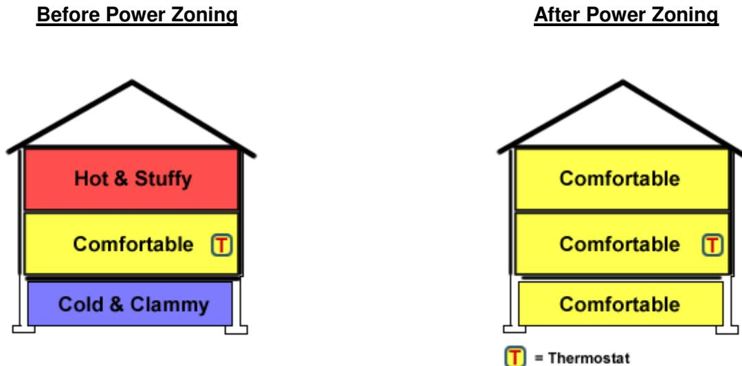
Figure 5 – Elimination of Stratification
